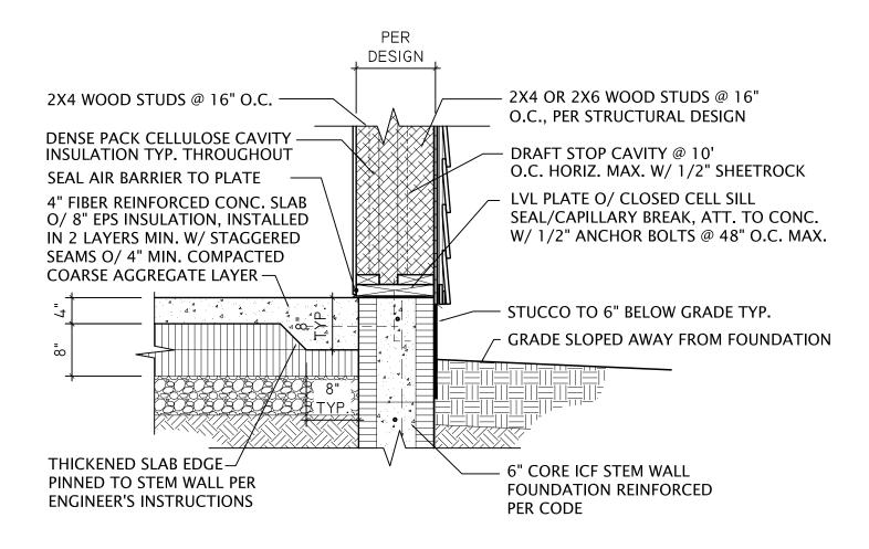
Double Stud Wall: Slab On Grade w/ Stem Wall
