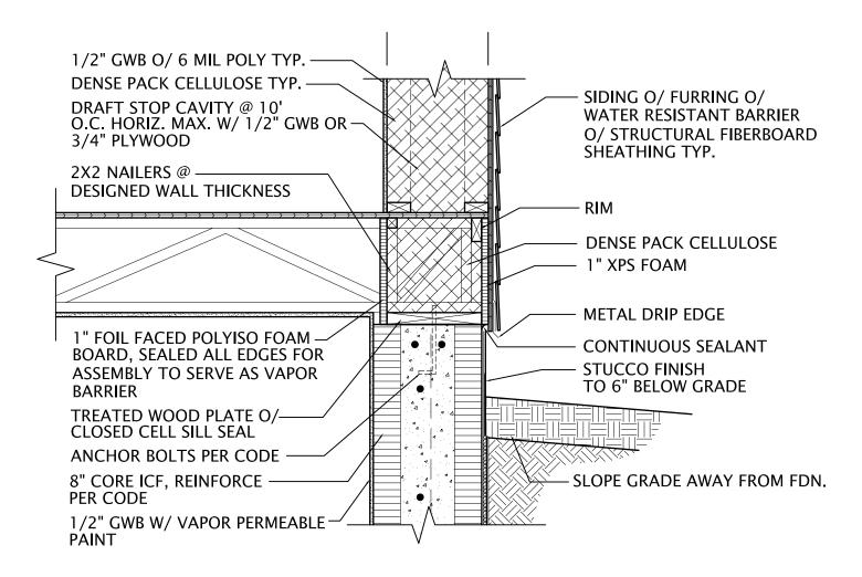
Double Stud Wall: Floor Truss to ICF Foundation
